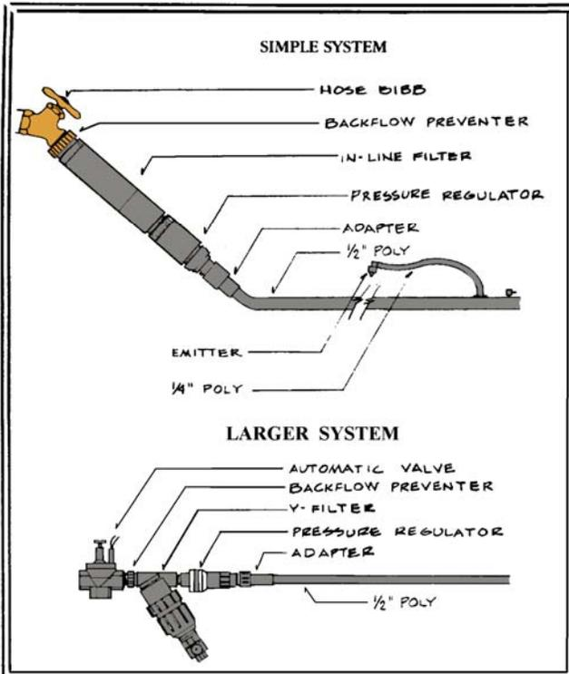
All these components are sized based on the expected flow of the system or zone.
